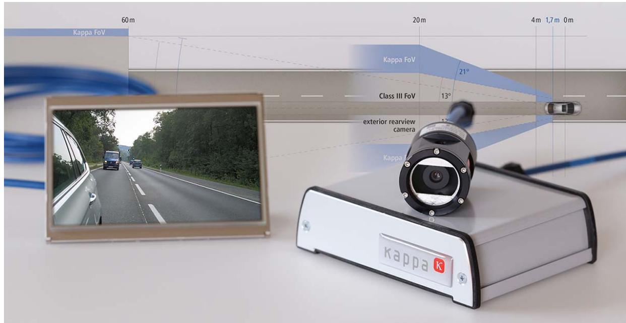
The flexible camera monitor system CMS HDR Mirror from manufacturer Kappa optronics has taken the lead position in the hypercar and super sports car market. The mirror replacement system consists of a camera, a controller, and a display. It combines state-of-the-art camera technology and expertise gleaned from numerous automotive projects. Its hardware and software were designed to comply with the ISO 26262 (ASIL B) functional safety standard.
